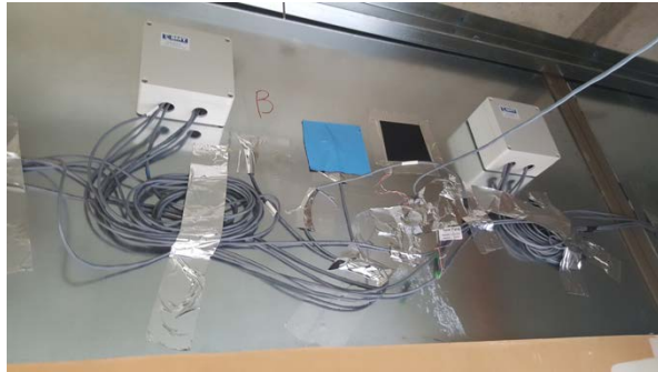
Figure 11. Typical data logger and sensor installation
