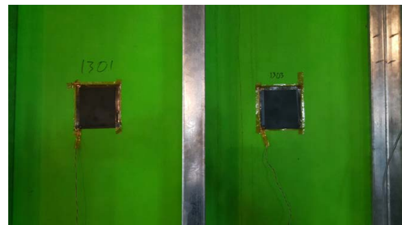
Figure 3. Interior Heat Flux Sensor Installation
