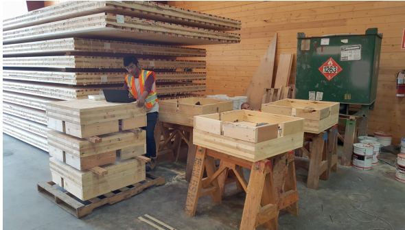
Figure 5. Six Additional Off-cuts Instrumented on May 27th, 2016
