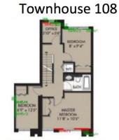
Figure 3: Sensors having elevated moisture content in the 2<sup>nd</sup> floor of Townhouse 108.
